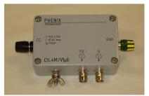
The CIL quadrupoles consist of an inductor in parallel with a damping resistor. The inductor and resistor are calculated to form, together with a high-voltage coupling capacitor, a second order high pass filter. Therefore, matching the range of the CIL with the size of the coupling capacitor with which it will be used is important.
