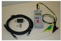
The instrument automatically synchronizes to line frequency by a photo diode. In case of insufficient pick-up of power frequency light, the calibrator automatically selects the internal quartz oscillator (50 Hz- and 60 Hz-versions available).
